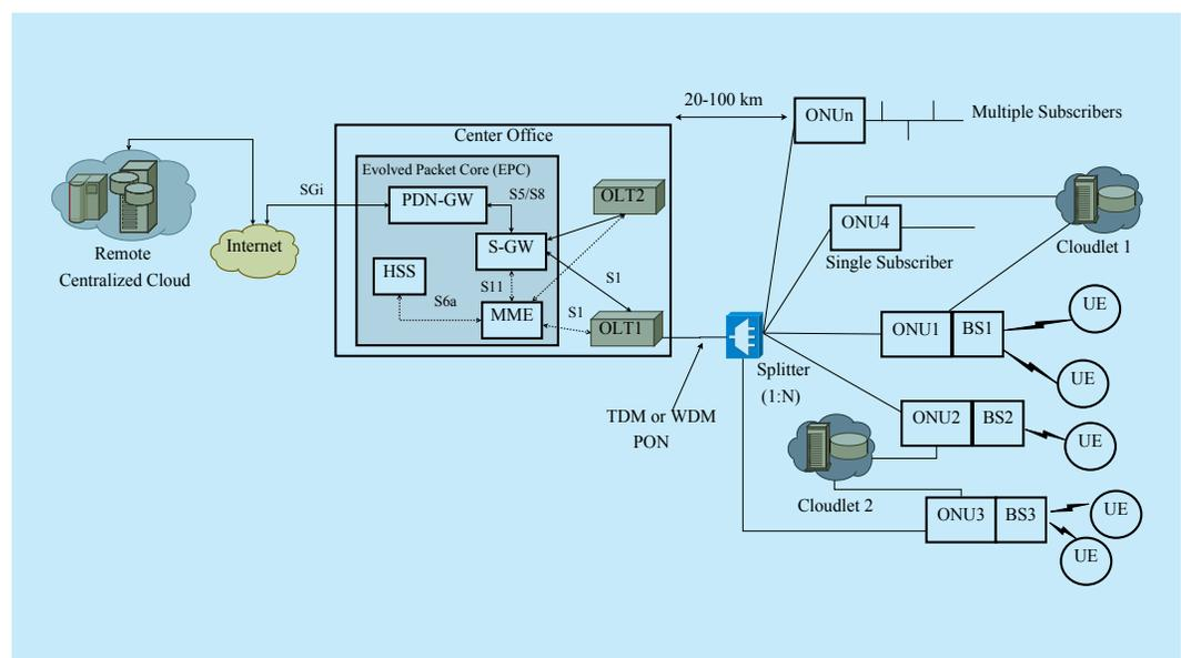
**Fig. 4** Cloud and cloudlet empowered FiWi-HetNet architecture.
