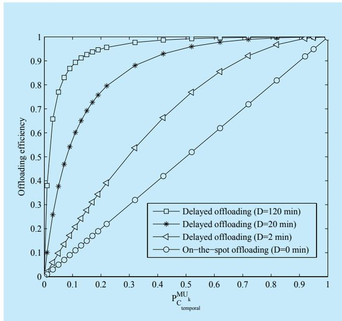
Fig. 2. Offloading efficiency vs. temporal FiWi connectivity probability of mobile users for on-the-spot and delayed offloading.
