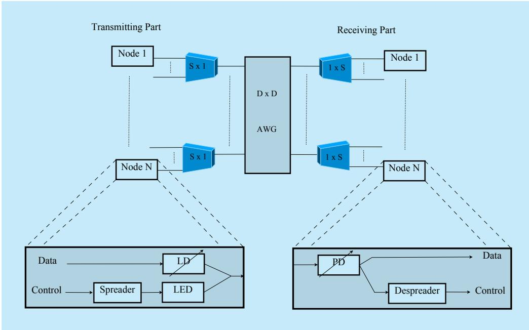
**Fig. 5** Scalable switchless single-hop WDM network using multiple FSRs of a wavelength-routing AWG for east-west flows in data centers.
